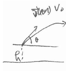
$$\vec{v}(0) = v_0 \cos \theta \vec{i} + v_0 \sin \theta \vec{j}$$
